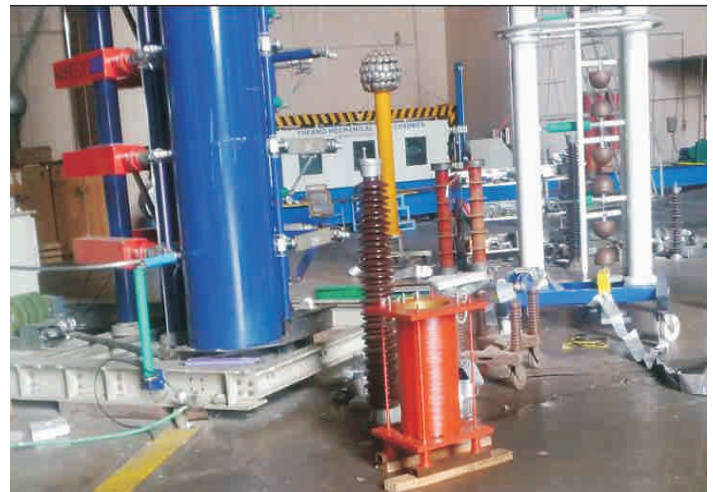
MSR Reactor coil being tested at CPRI
